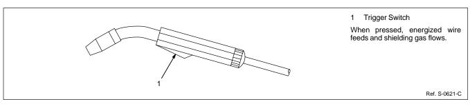
Figure 4-1. Using Gun Switch
